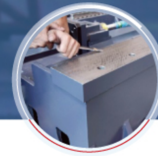
6 Scraping of Joint Surface of Bed and Column
