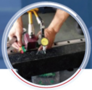
2 Linear Guideway Align
